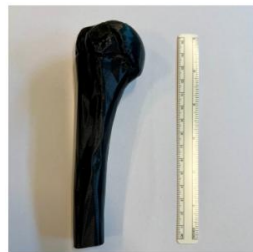
3D printed Bone inside Phantom
