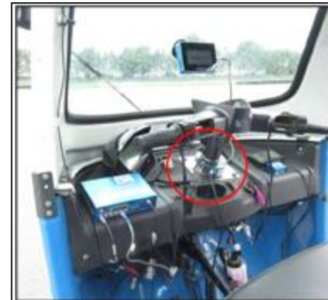
RT1003 IMU and Steering sensor for Vehicle dynamics Parameter Measurement
