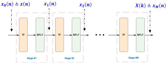
In the ideal BFP-FFT a scale down at stage m will happen iff one of the stage's outputs is larger than 1 (re-calculation is required)
