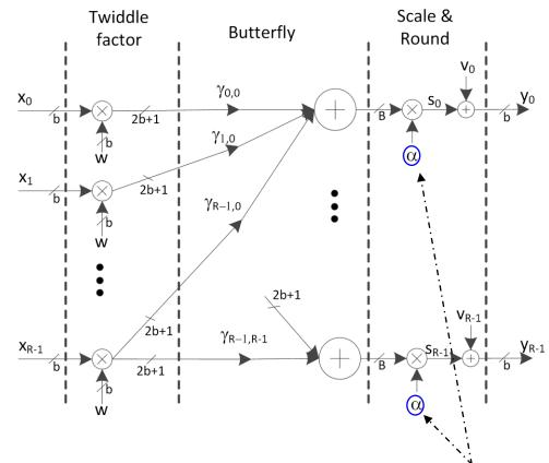
• The output of the butterflies are scaled down (by right shift,  $\alpha = 2^{-q}$ ) and rounded before stored to memory
