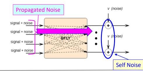
Noise generated at 1<sup>st</sup> stage propagates to the output through M-1 following stages Results in accumulation of  $R^{M-1}$  noise sources
