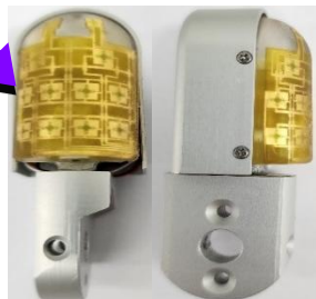
Artificial fingertip with tactile sensor
