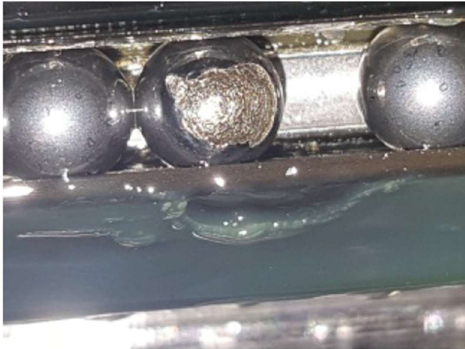
Figure 1: Figure presenting a pitting damage to a ball rolling element at LWM.
