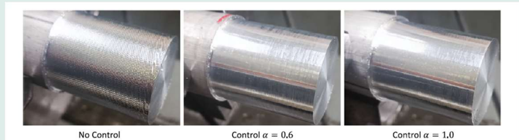
Fig. 15. Appearance of workpieces after machining, with and without control.
