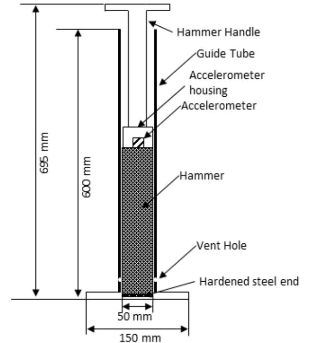
Construction of a Clegg Impact Hammer used for measuring Penetration resistance
