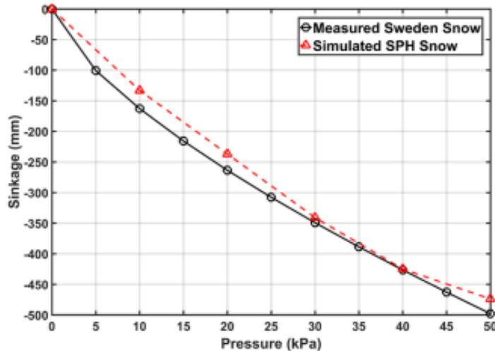
Calibration results for simulated and measured snow: (a) pressure–sinkage results\*\*
