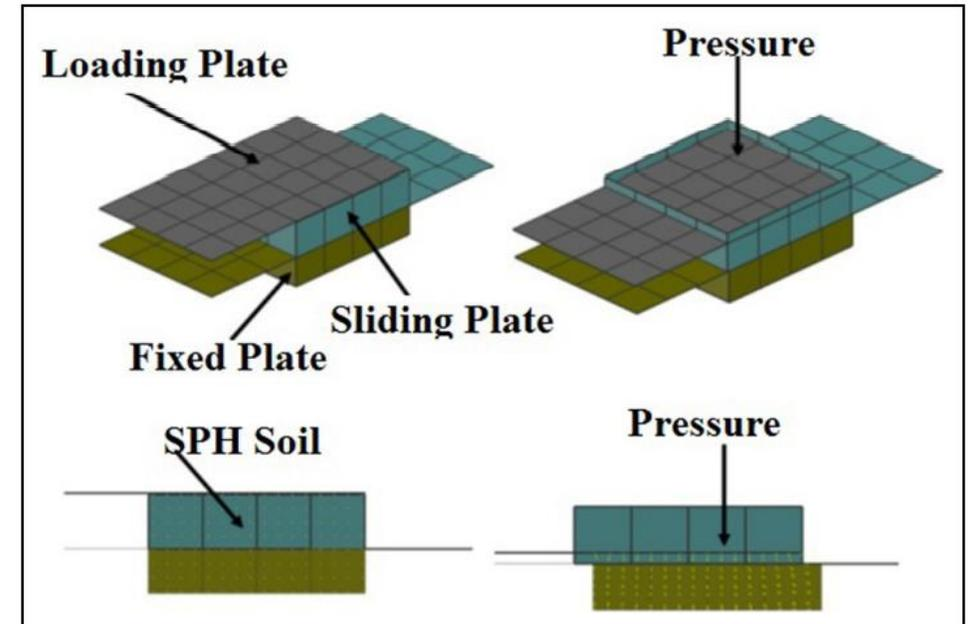
Shear–strength test with SPH snow
