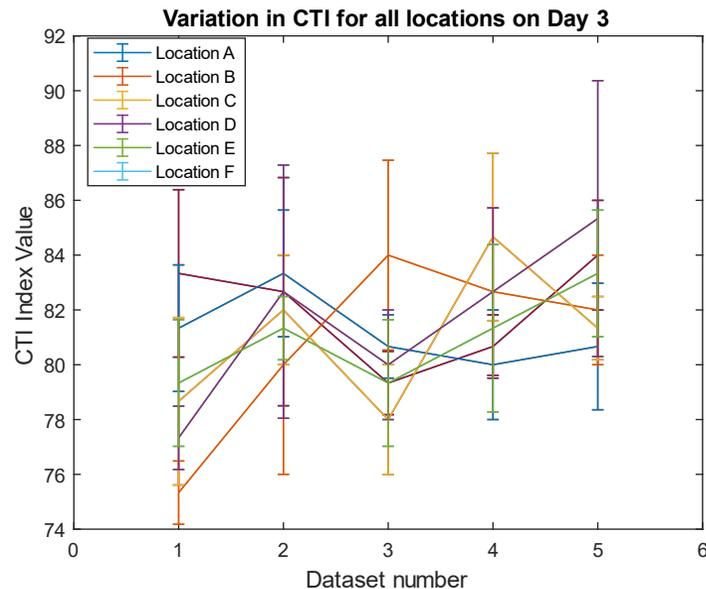
Plot of the mean and standard deviation of measured values of CTI Penetrometer on day 3
