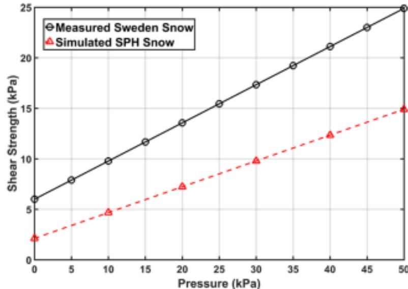
Calibration results for simulated and measured snow: shear–strength results\*\*
