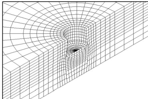
Drucker-Prager cap with vertical shear contact surface
