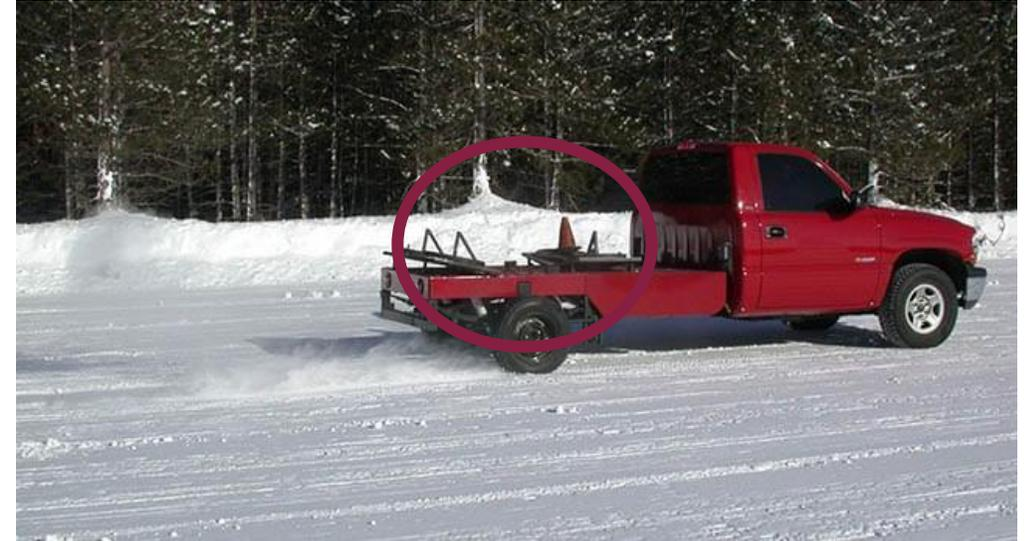
Instrumented traction truck used for ASTM F1805 testing of winter tires. Courtesy: [Smithers: Snow and Ice Traction](#)
