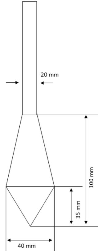
Construction of Rammsonde penetrometer
