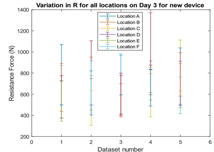
Plot of the mean and standard deviation of penetration resistance to new device
