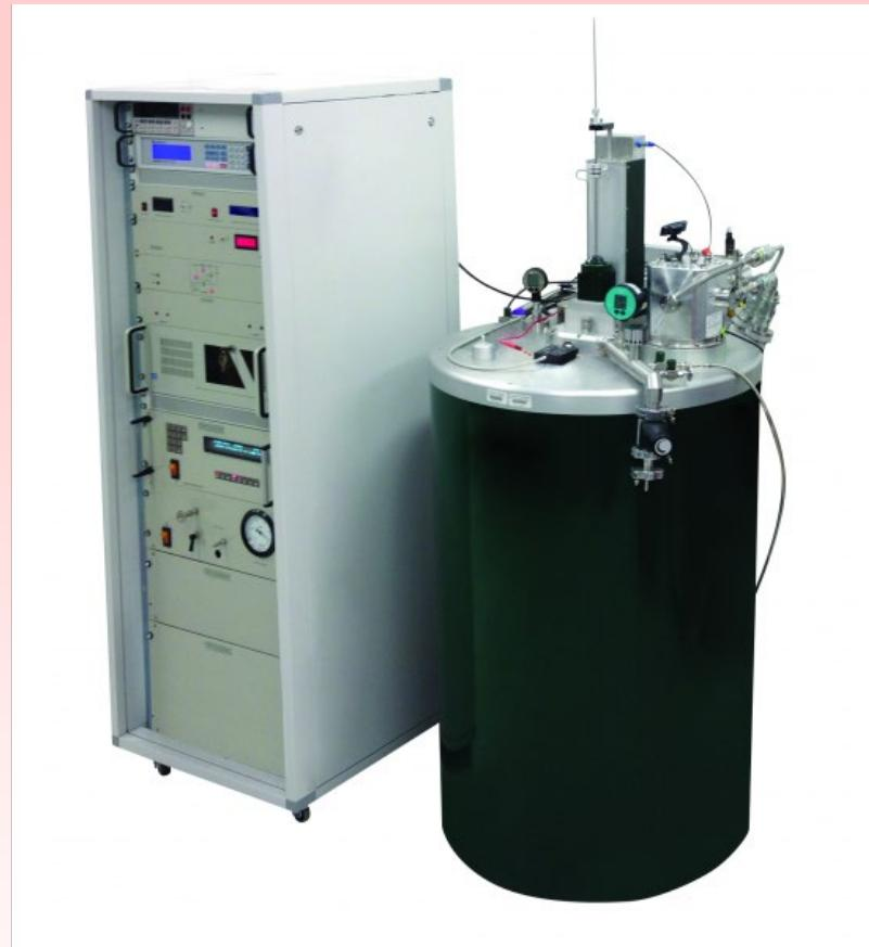
SQUID (superconducting quantum interference device)
