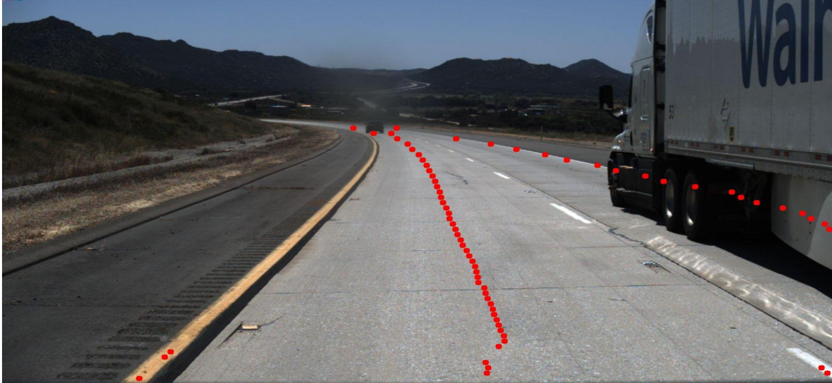
Figure 18: False positive lane detection causes unsafe driving
