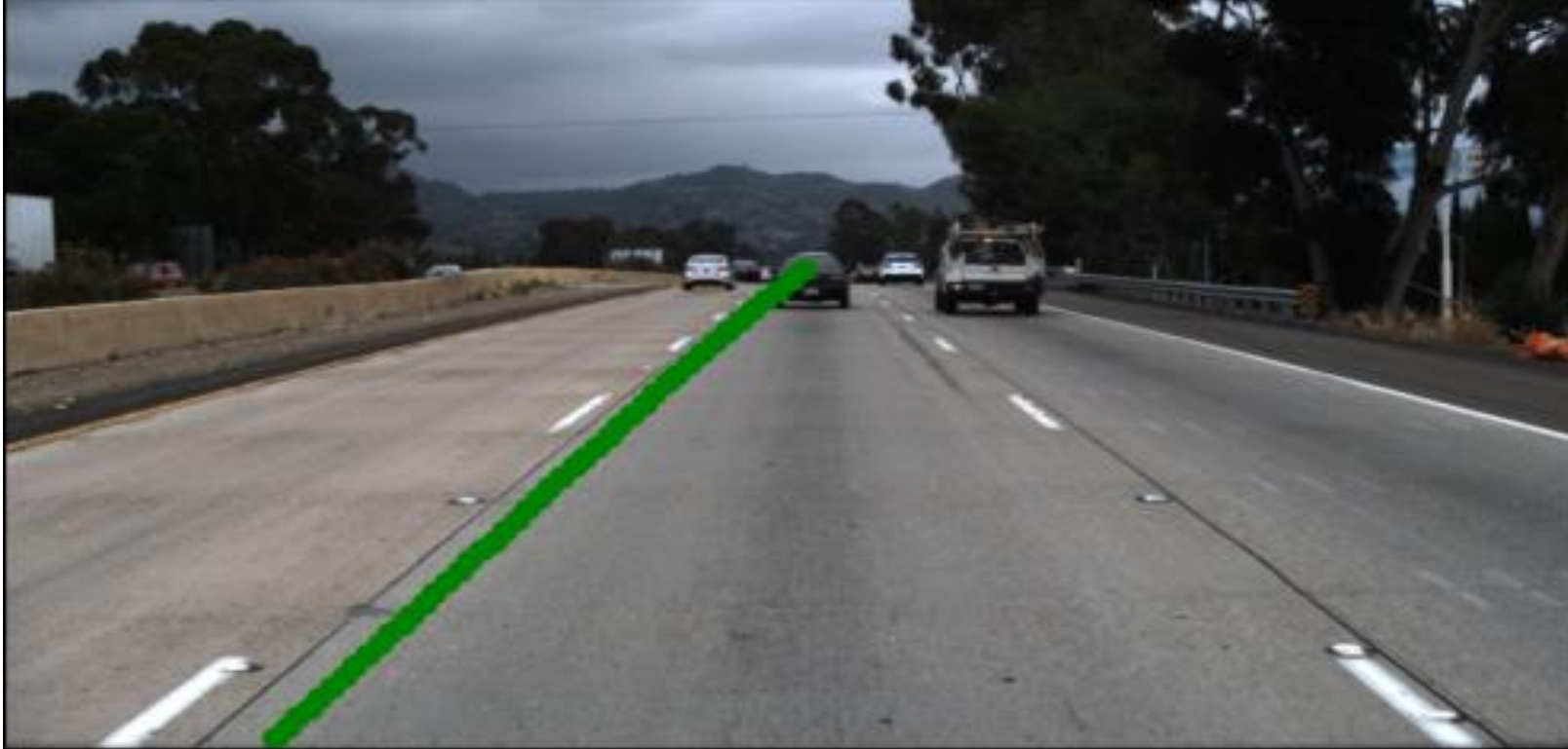
Figure 19: Driving scene illustrating the problem with the lane abstraction approach
