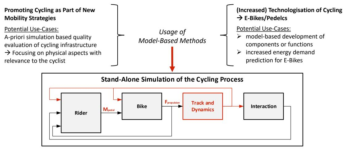
→ Resulting dynamics define the physical model structure of bike and rider subsystems
