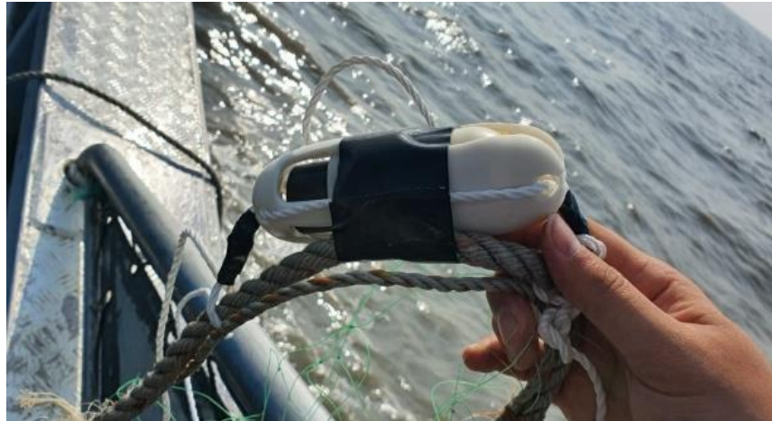
Fig. 8: Underwater acoustic tag used in the test
