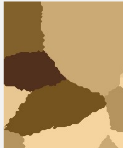
Macrostructure after heating the sample to the nominal test temperature of 1450°C and cooling at 1° C / s („hot” grips, S355 grade steel)
