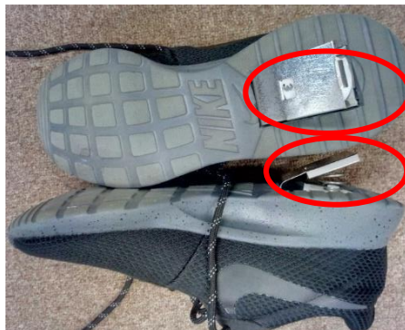
Prototype of the gait assist shoes with the simple heel-raising unit
