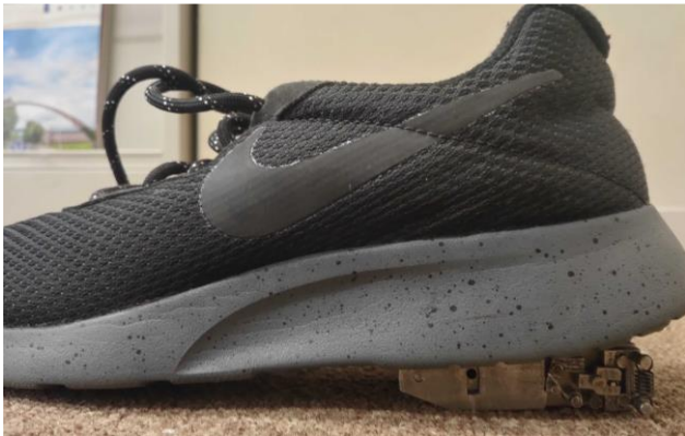
(b) Shoes: Spring compressed state
