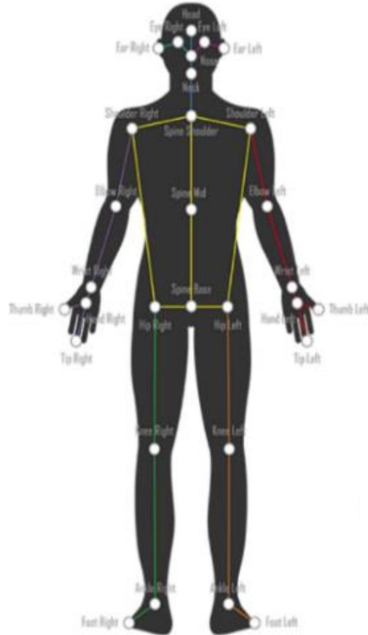
Fig.4 Skeletal coordinate positions that can be detected by VisionPose
