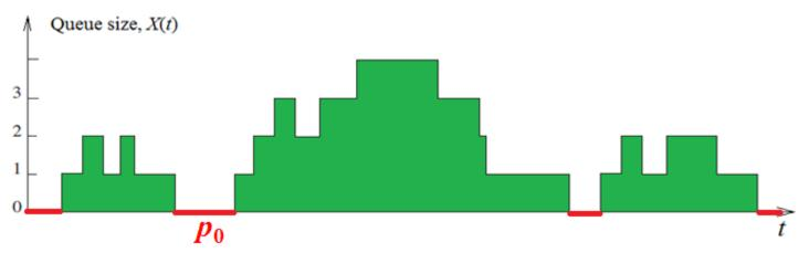
• # of packets sent in a long interval of length T is:  $(1-p_0)T\mu$
