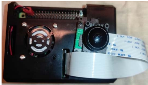
Raspberry Pi with a camera sensitive to several spectrums
