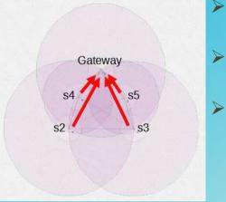
In the star topology every sensor node, marked as s2 to s5, is connected to the gateway and sends data directly to the gateway.
