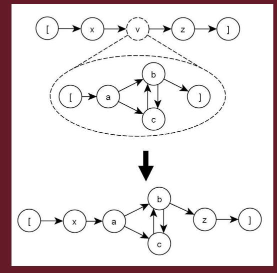
Refinement of a vertex v and its embedding in the refined ESG
