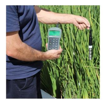
DO was measured with a probe HI98198 optical meter (HANNA).
