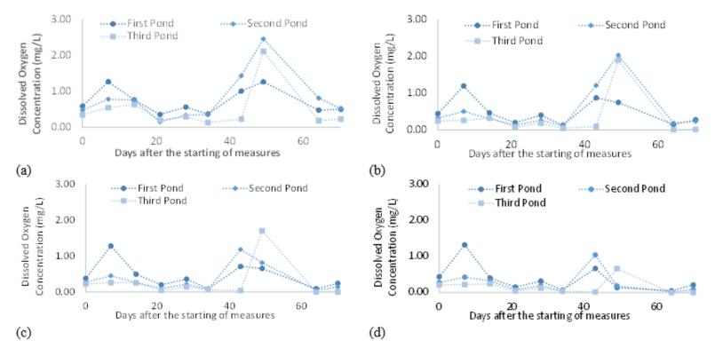
Figure 3. Overview of DO concentration at different depths (a) 6 cm, (b) 25 cm, (c) 50 cm, and (d) 75 cm.
