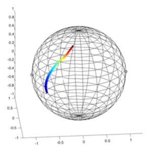
Fig. 1. A Poincare' Sphere showing an RF signal fingerprint varying from red to blue frequency.
