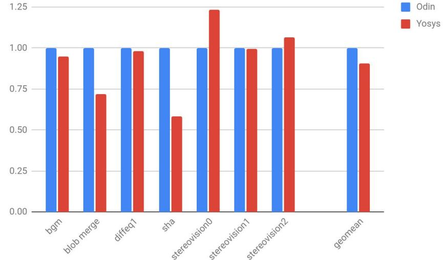
*Normalised logic area used for Odin-II vs Yosys flow for benchmarks with >1000 blocks*
