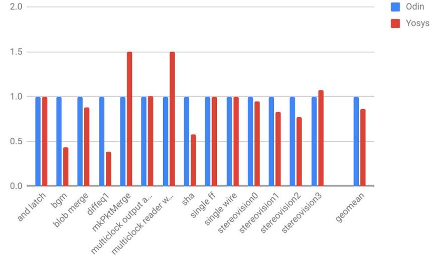
*Normalised critical path delay of Odin-II vs Yosys flow*
