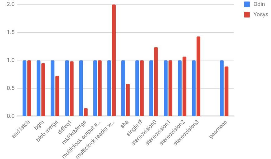
*Normalised logic area used for Odin-II vs Yosys flow*
