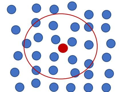
Nodes inside the red ring is covered by the transmission form the red node.
