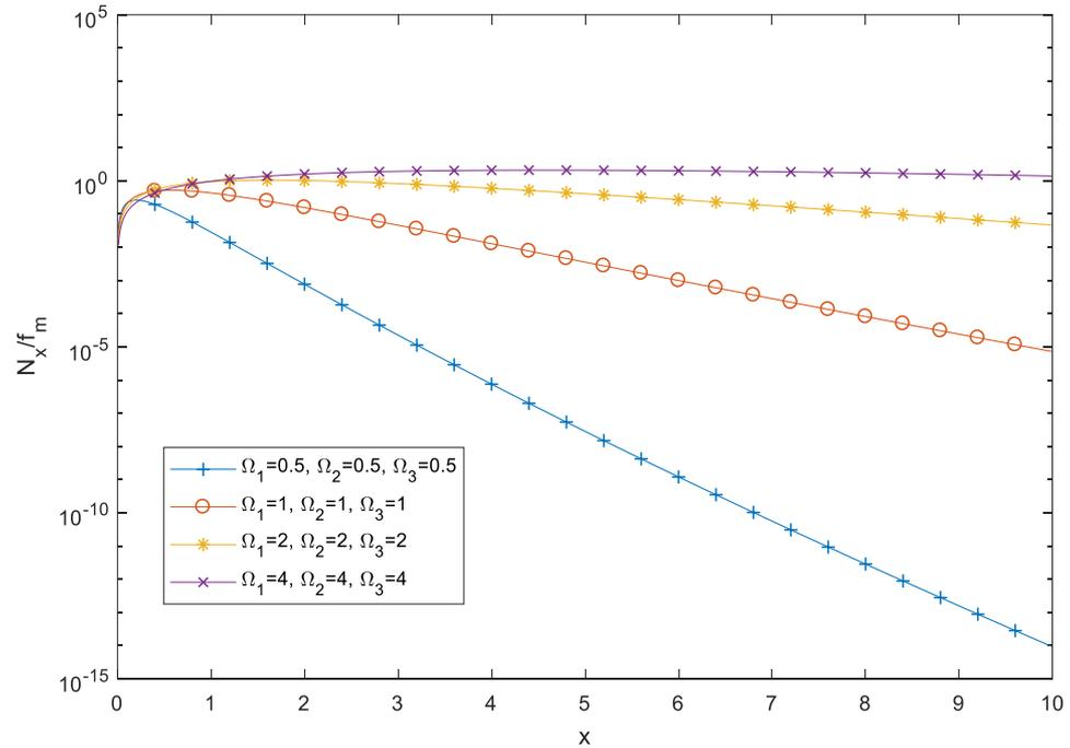
► Fig. 5 LCR normalized by  $f_m$  versus signal envelope  $x$  for various values of signal powers  $\Omega_i$
