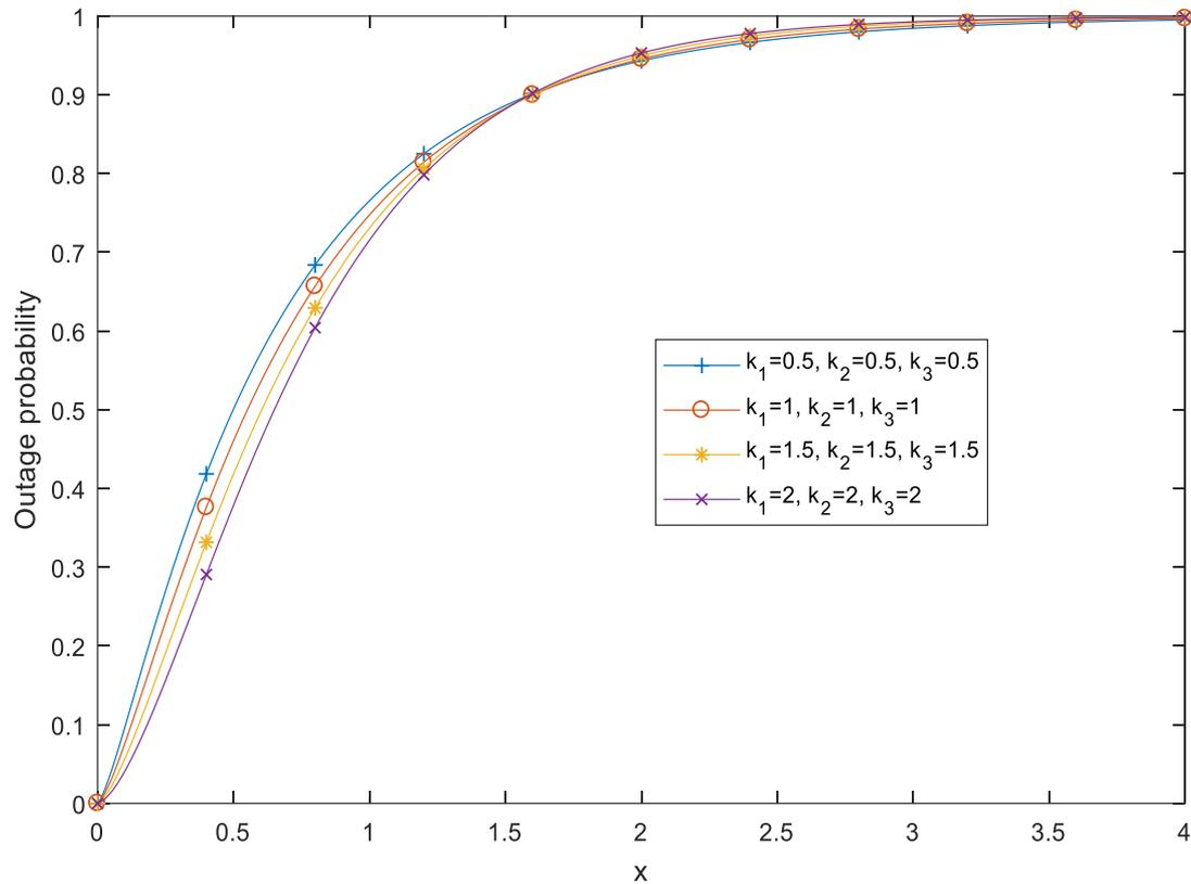
► Fig. 2 Outage probability of product of three Rician RVs versus signal envelope  $x$  for different values of Rician factor  $\kappa_1$  and signal power  $\Omega=1$
