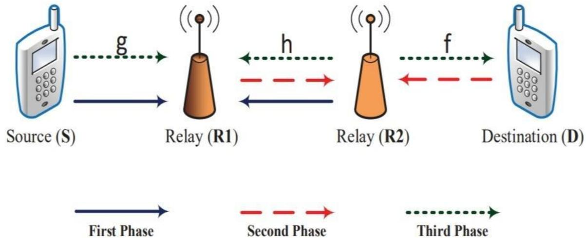
► Fig. 1 System model of a three-hop wireless relay.
