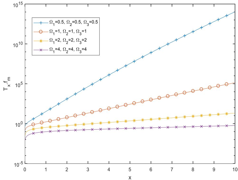
► Fig. 7 AFD normalized by  $f_m$  depending on signal envelope  $x$  for  $\kappa=1$  and different values of signal powers  $\Omega_i$
