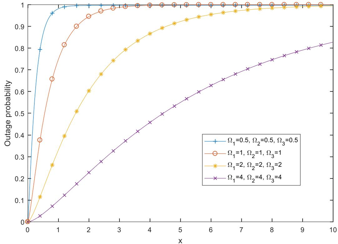
► Fig. 3 Outage probability of product of three Rician RVs depending on signal envelope for different values of signal power  $\Omega_i$  and Rician factor  $\kappa=1$
