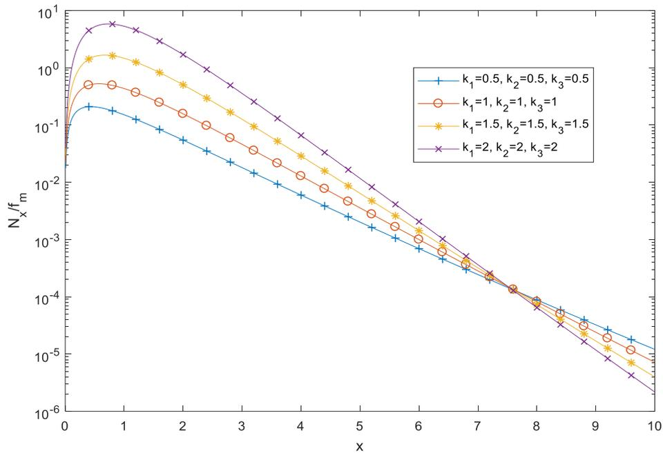
► Fig. 4 LCR normalized by  $f_m$  depending on the signal envelope  $x$  for various values of Rician factor  $\kappa_i$  and signal power  $\Omega=1$
