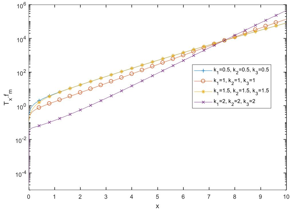
► Fig. 6 AFD normalized by  $f_m$  versus signal envelope  $x$  for different values of Rician factor  $\kappa_i$  and signal powers  $\Omega_i=1$
