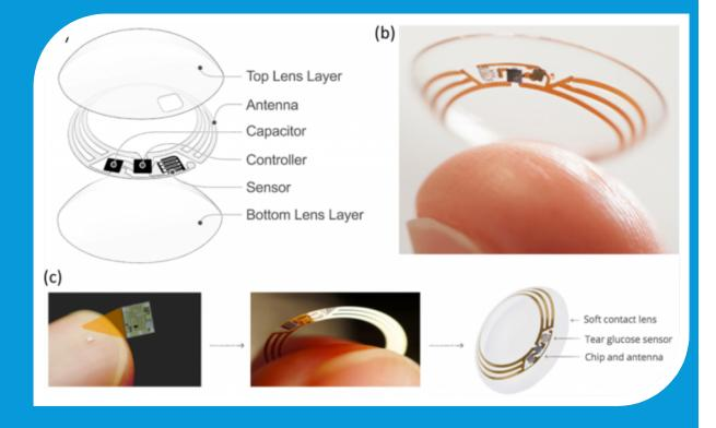
• **Google Lens**, in collaboration with Novartis, proposes a contact lens that contains a microchip that measures blood glucose directly from the tear fluid and transmits information to a mobile device;
