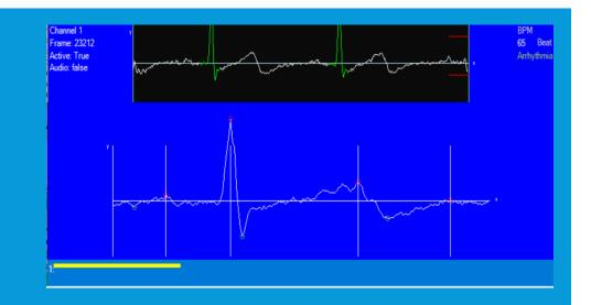
For processing and filtering graphics, there were used two filters. Haar filter used in mathematics for waves, form a wavelet family. Wavelet analysis is similar to Fourier analysis, because it allows a target function to be represented as an orthonormal basis. Using the wavelets for Electrocardiography representation is quite useful if the sampled signal is continuous and has sudden transitions
