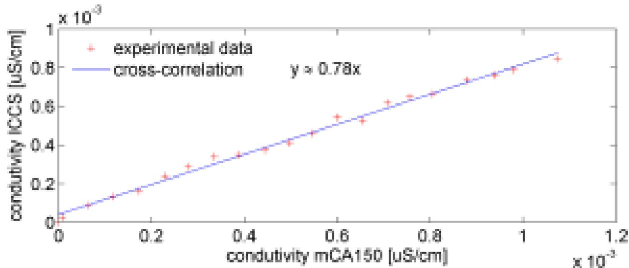
Calibration curves and comparison of measurements of the electrical conductivity from experimental solutions obtained with the intelligent and customized sensor with cell constant of  $0.255 \text{ cm}^{-1}$ .
