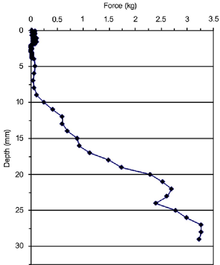
Soil resistance variations to the root penetration in function of depth Z and coordinates X and Y.
