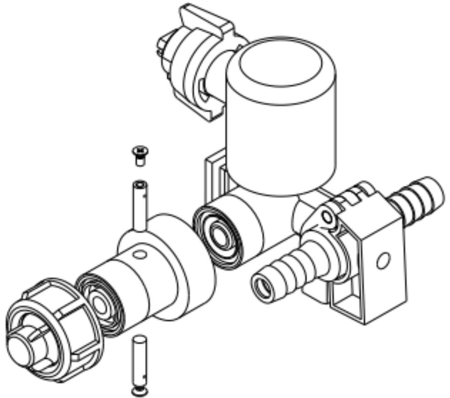
**Details of the smart sensor customized to measure the response time of a system of direct injection of pesticides.**
