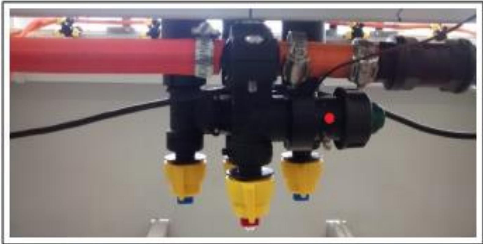
Instrumental arrangement for validation of the intelligent sensor to measure response time of a direct injection sprayer with TeeJet® QJS Multiple Nozzle Bodies e-ChemSaver.
