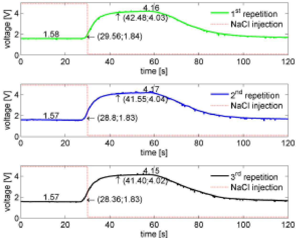
Transients and transport delay times of the sprayer with the conductivity sensor assembled in an actual spraying system with water-NaCl solution flow of  $16 \text{ l/min}$  and pressure equal to  $200 \text{ kPa}$ .
