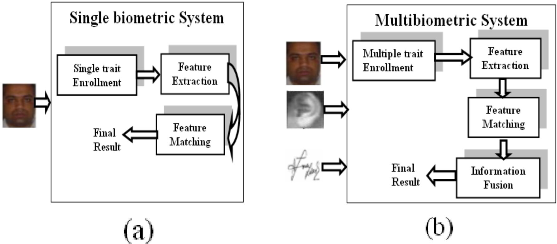
Fig. Block diagram of two biometric systems (a) single biometric (b) multibiometric
