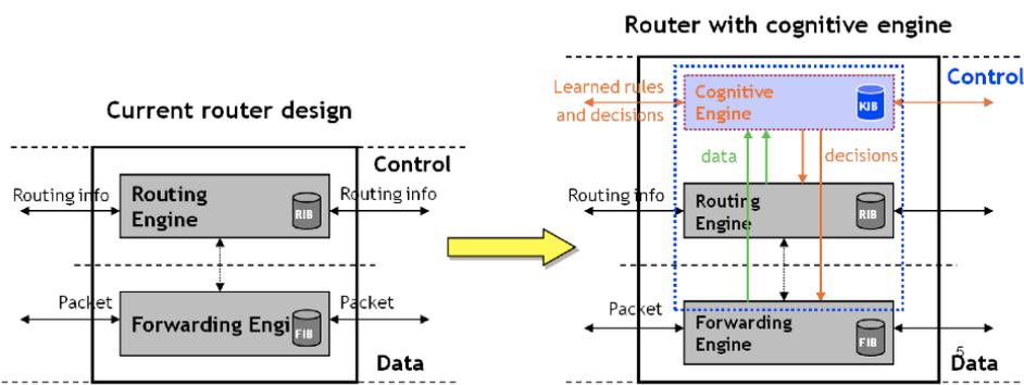
A cognitive routing system according to FP7 ECODE (Experimental Cognitive Distributed Engine)
