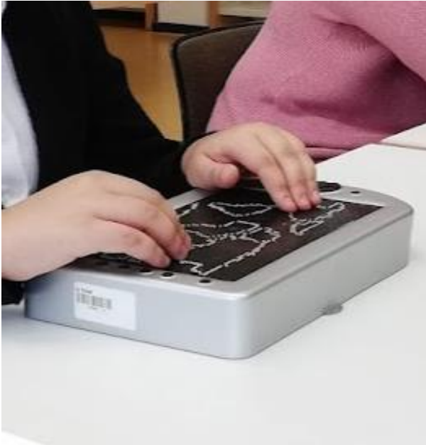
Figure 1: Audio-tactile representation of the world map on a Metec pad. Own representation.
