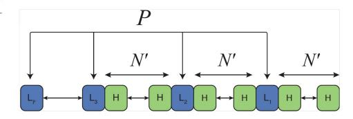
Illustration of detection probe (packet train) constructed by ConstructLProbe-Sequence function. *N*' is the number of packets in the *separation packet train*. *P* is the total number of *priority packets*. (Green) High priority packets. (Blue) Low priority packets. The Algorithm 3 demonstrates the creation of the LProbe specified in the above figure. HProbe is constructed in a similar fashion.
