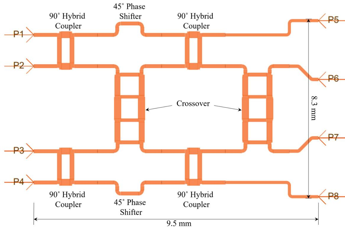
Fig 9. Layout of microstrip  $4 \times 4$  Butler Matrix in ADS.
