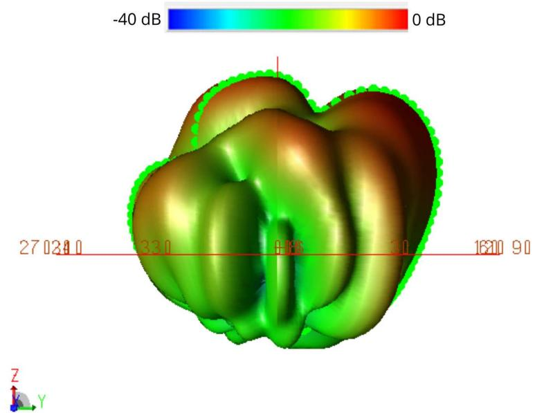
Fig 18. 3D beamforming when Port 2 is excited.
