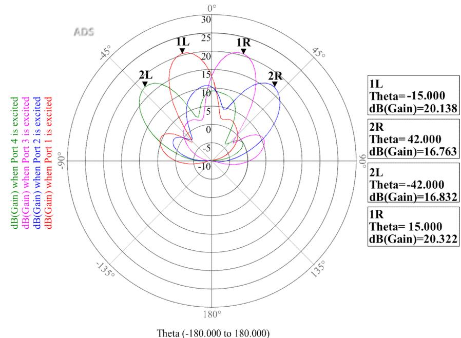
Fig 14. Polar plot of beamforming by the designed  $4 \times 4$  Butler Matrix.
