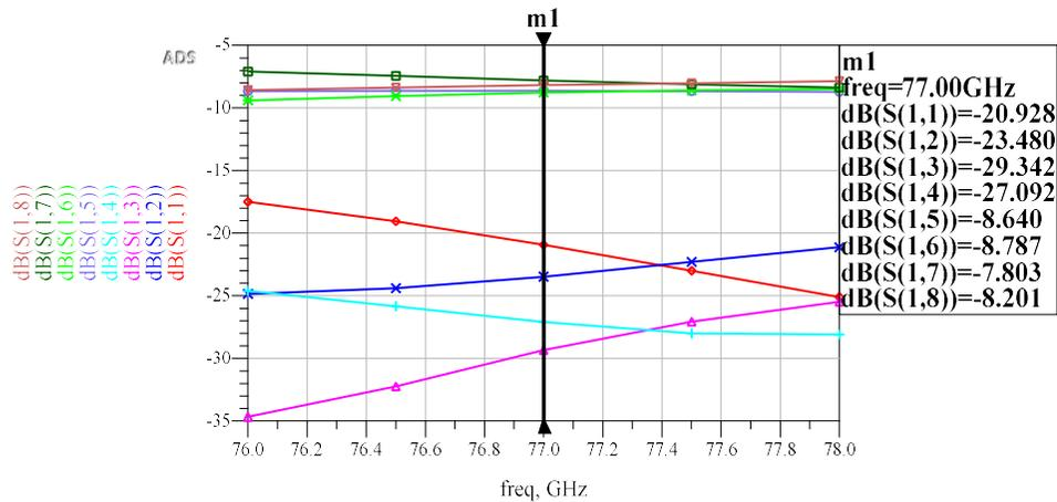
Fig 10. Simulation result of microstrip  $4 \times 4$  Butler Matrix when Port 1 is excited.
