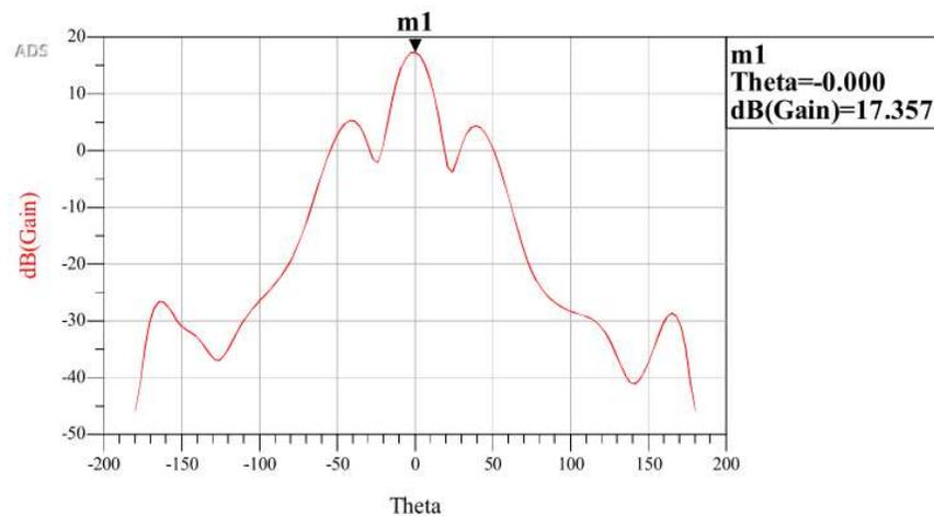
Fig 15. Rectangular plot of beamforming by the designed  $4 \times 4$  Butler Matrix.
