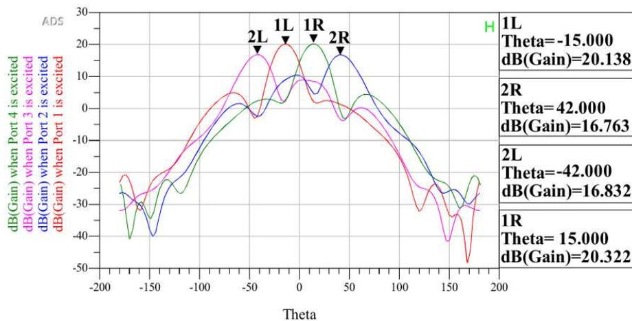
Fig 13. Rectangular plot of beamforming by the designed  $4 \times 4$  Butler Matrix.
