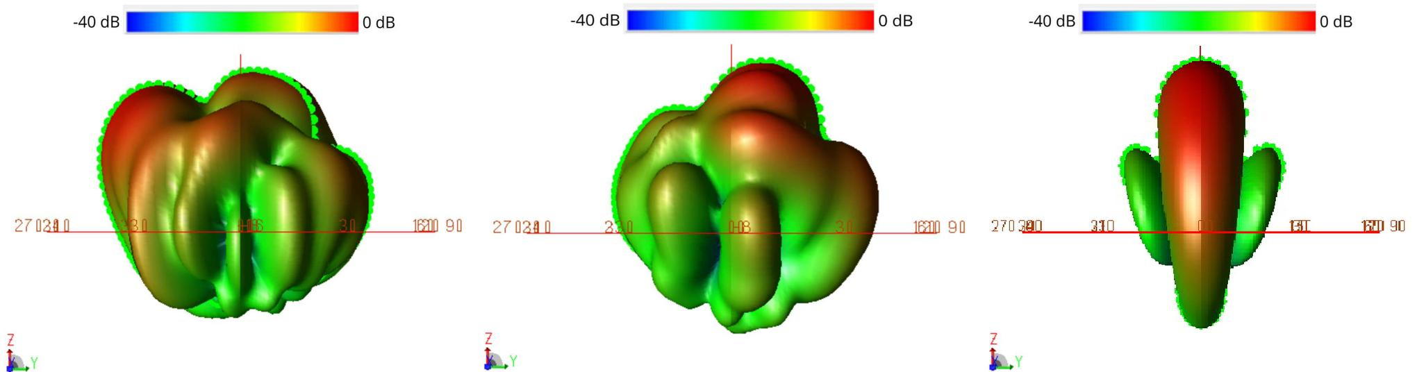
Fig 19. 3D beamforming when Port 3 is excited.
