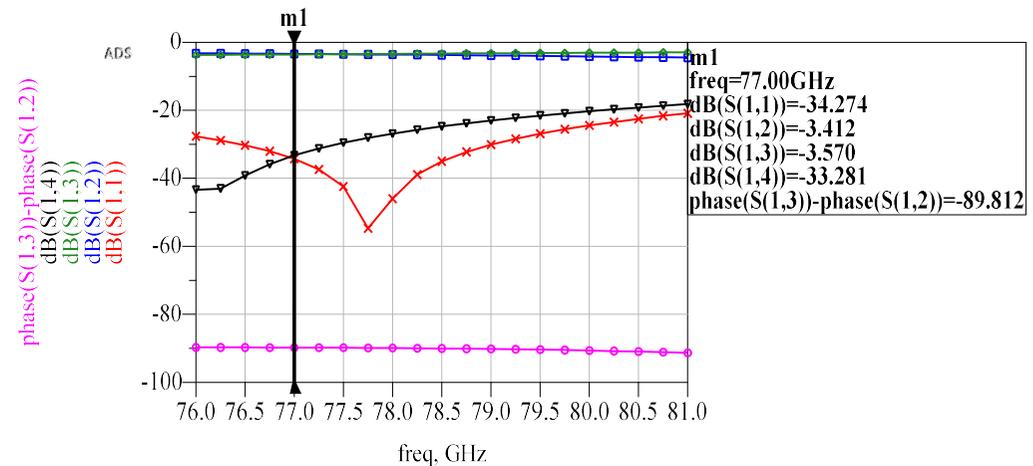
Fig 4. Performance of microstrip 90° hybrid coupler.
