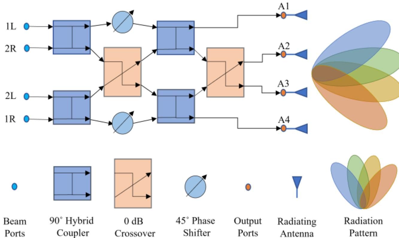
➤ It has four input ports and four output ports.
