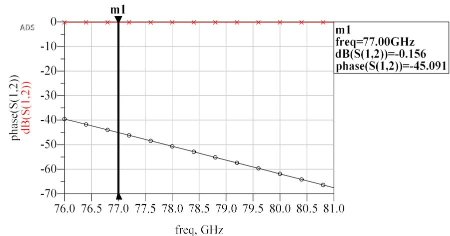
Fig 8. Simulation result of microstrip 45° phase shifter in ADS.
