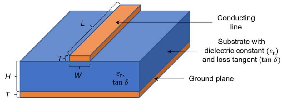
Fig 2. Microstrip line geometry.
