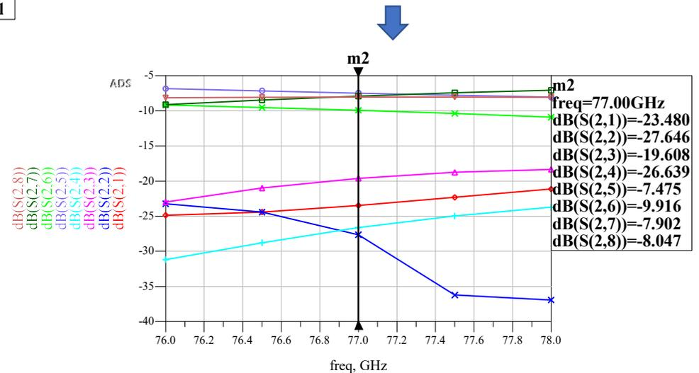
Fig 11. Simulation result of a microstrip  $4 \times 4$  Butler Matrix when Port 2 is excited.
