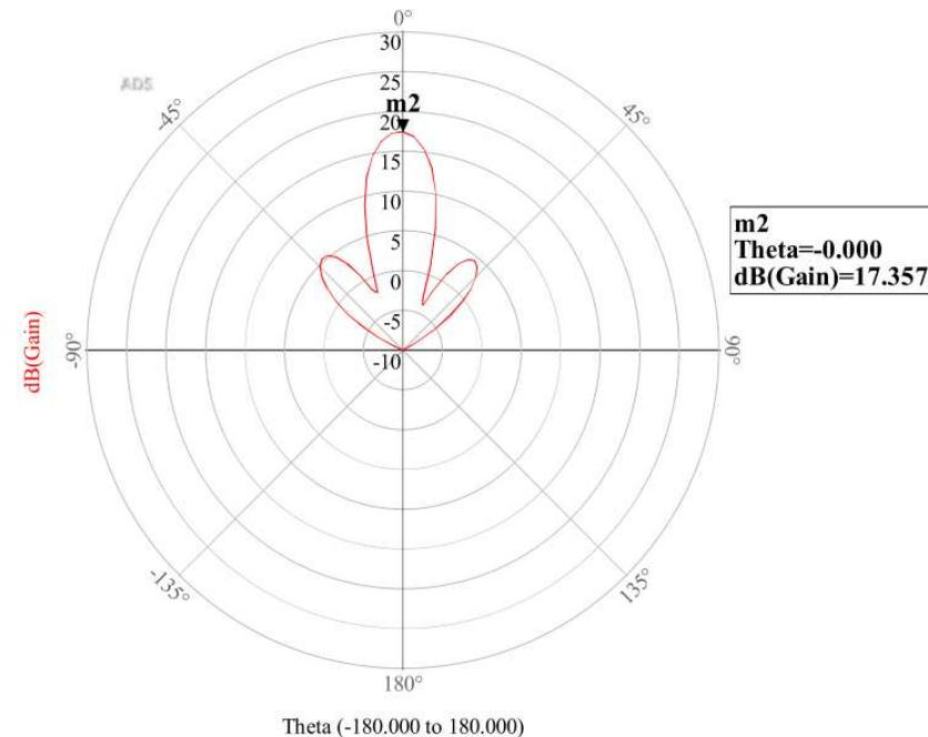
Fig 16. Polar plot of beamforming by the designed  $4 \times 4$  Butler Matrix.
