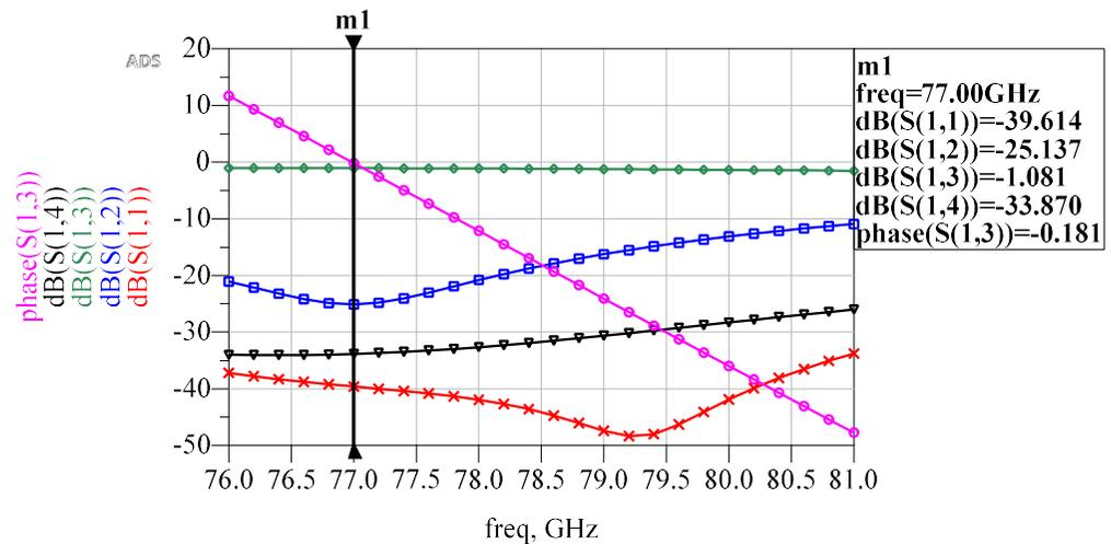
Fig 6. Simulation result of microstrip crossover in ADS
