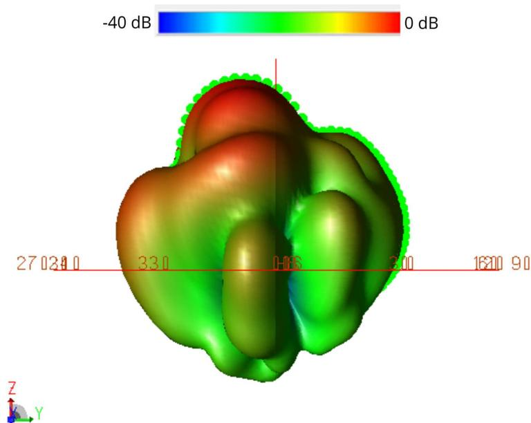
Fig 17. 3D beamforming when Port 1 is excited.
