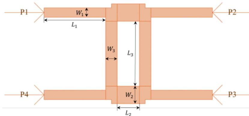
Fig 3. Layout of microstrip 90° hybrid coupler.
