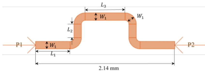
Fig 7. Layout of microstrip 45° phase shifter
