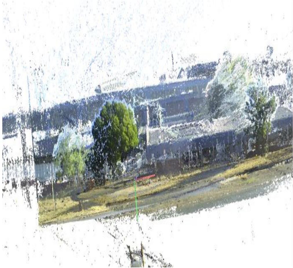
Figure 7. Denser point of cloud with multiview stereo.
