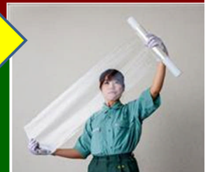
CNF Transparent sheet developed by Oji Holdings & Mitsubishi Chemistry
