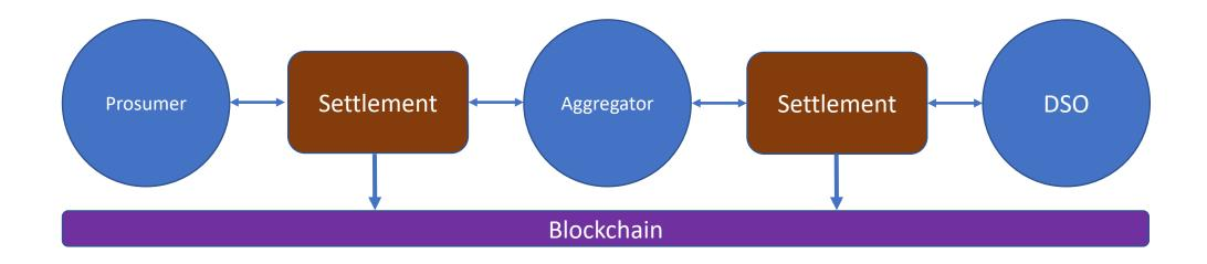
This figure shows the settlements between the prosumers and the aggregator, and the aggregator and the DSO. The transactions are written to the blockchain
