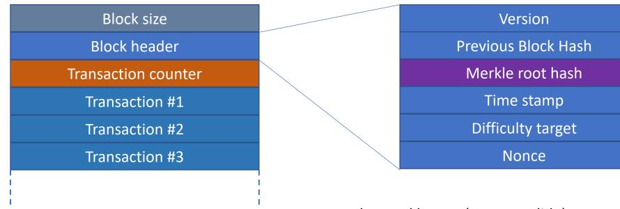
The Merkle tree (see next slide) ensures the integrity of each transaction added to a block
