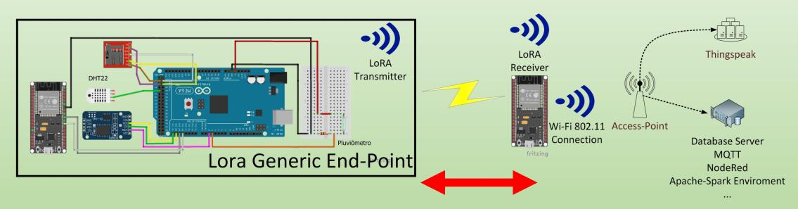
Receiver Wi-Fi LoRa module was positioned 500 meters away playing the role of a gateway
