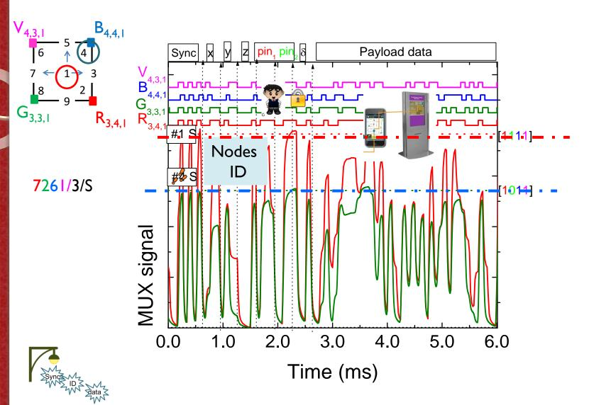
The footprint position comes directly from the synchronism block, where all the received channels are, simultaneously, *on* or *off*.
