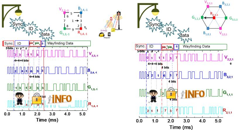
Cell's IDs and passwords are encoded using a 4 bits binary representation for the decimal number.
