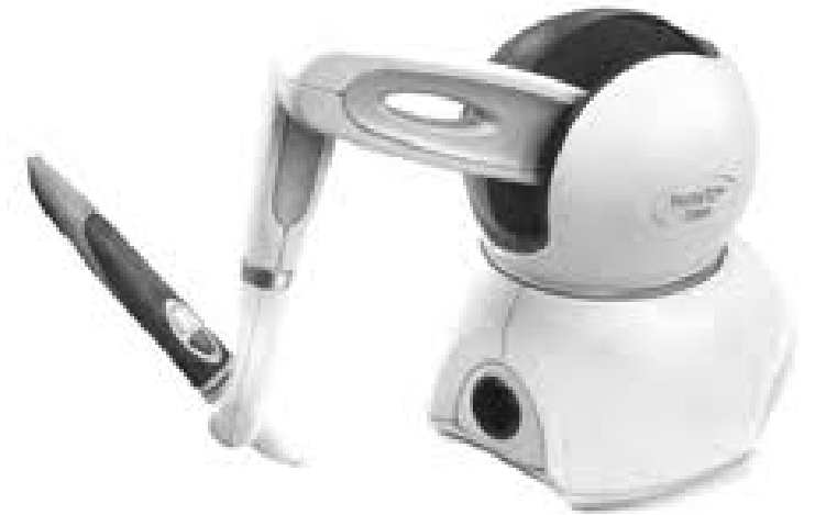
Phantom Omni (above) and Novint Falcon are the primary sources of haptic feedback for handwriting training.
