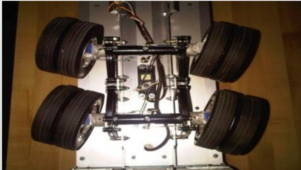
A small-scaled LCV with active trailer steering system [7]
