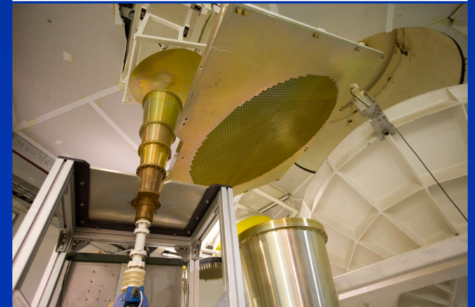
Fig. 2-12. Goldstone 70-m antenna XTR cone X-band HEMT amplifier.
