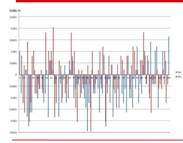
Chart shows differences between two AMR sensitivity amplitude measurements with an interval of one day for 100 AMR devices on a silicon wafer with a standard deviation of 0.9mV.
