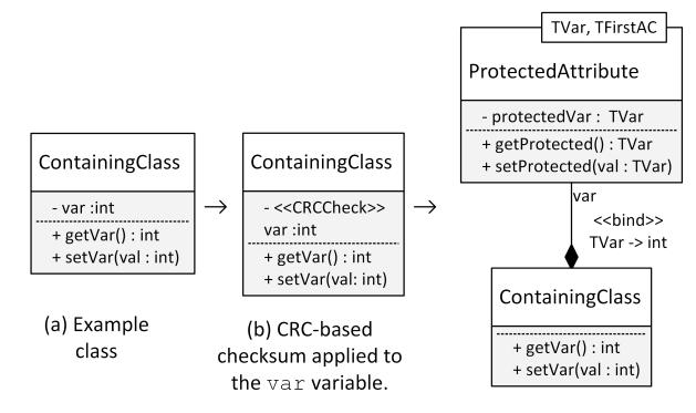
(c) Primitive var variable replaced by wrapper class (ProtectedAttribute) that contains a CRC-based error detection mechanism.
