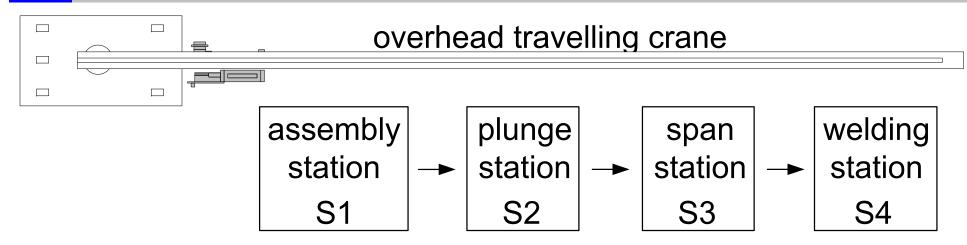
Overhead travelling crane lifts a filter basket out of a station, transports it to the next station and **inserts it directly** in this station. This is just possible if this station is free.
