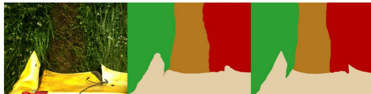
Image for segmentation of areas of cut grass (left), test mask (middle), ground truth map (right); standing meadow in green, grass turf in dark brown, machine in light brown and mown grass in red
