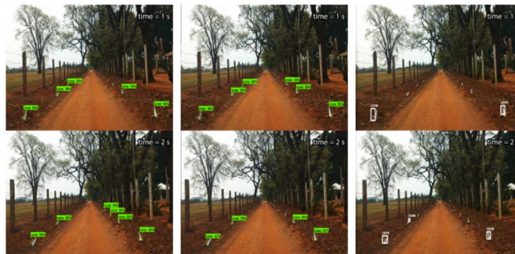
Comparison of detection methods: Faster R-CNN (left), SSD300 (middle) and Fast YOLOv2 (right)
