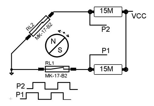
P1 – Basic contact P2 – Direction contact
