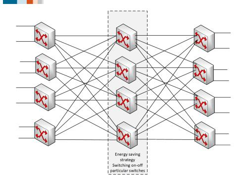
In the case of low network load it is possible to disable the switches of the middle section.
