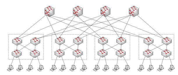
Switching network (switching fabric) is a combination of hardware and software that controls traffic to and from a network node with the use of multiple switches
