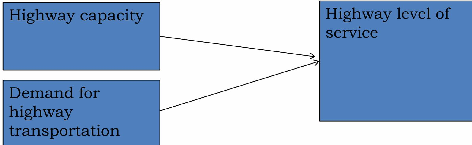
*Level of service A: Free flow speed, freely change lanes. Spacing > 25 car lengths.*
