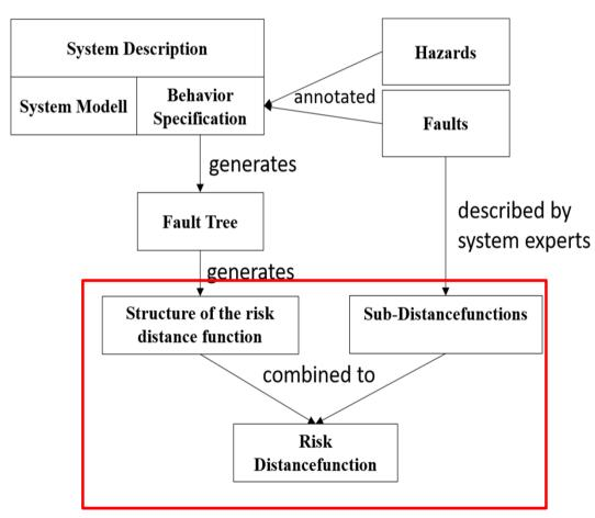
Use of the system and behavioral description including annotated hazards and causes to create the risk distance function
