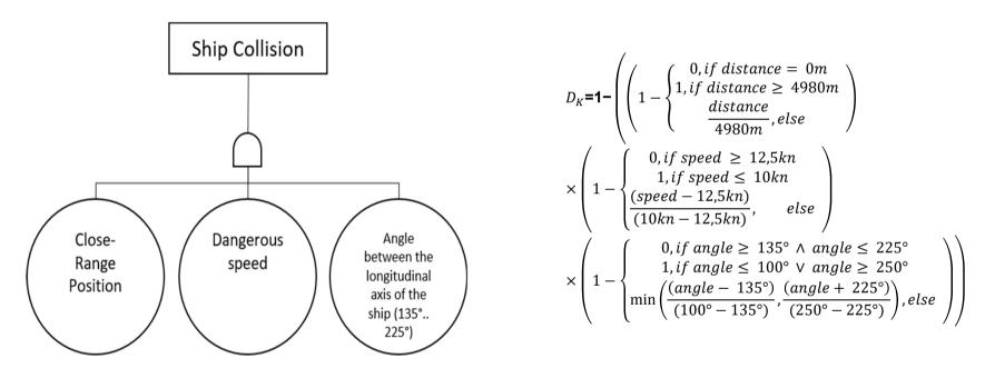
Simple Fault Tree for a frontal collision between two ships and the corresponding risk distance function
