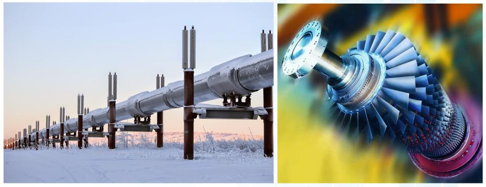
Pipeline, Alaska Temperature < -50°C, humidity, condensation, extreme geographical localization Turbines Temperature > 500°C, Rotation speed (26000 rpm), magnetic fields and metallic environment
