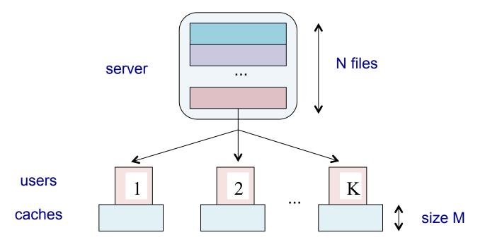
Load of shared link using **uncoded** caching: K(1 - M/N)
