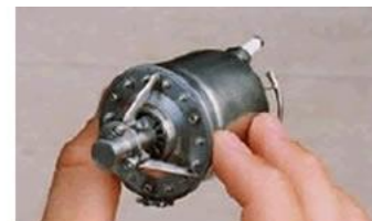
Micro gas turbine
