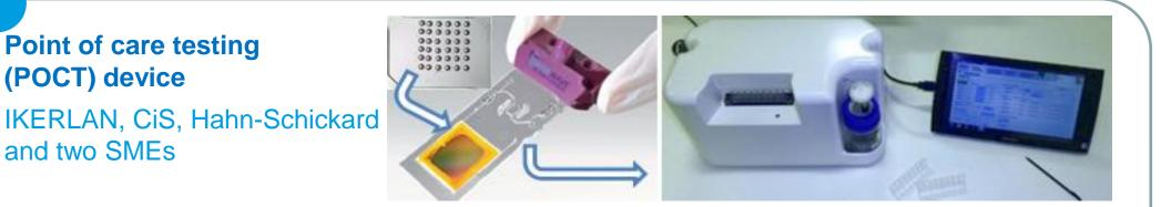
Modular system for multi-parametric optical detection using an automatised biological protocol. First validation by detection of several microtoxins
